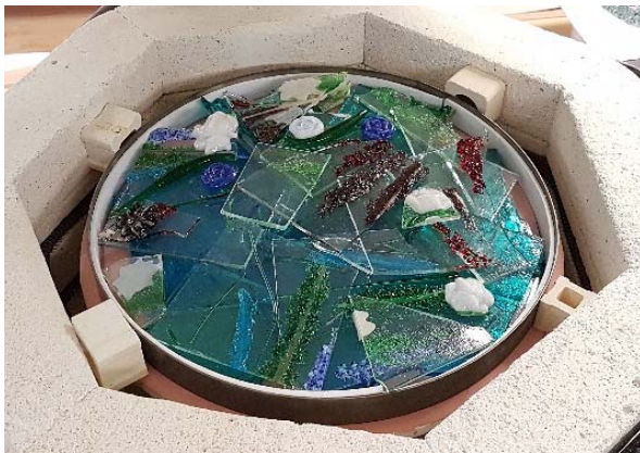
Glass project blocked in place in the kiln ready to be combed.
