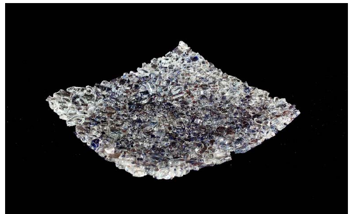
Tempered glass tray with float compatible frit
