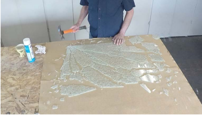
Tempered glass broken into chips
