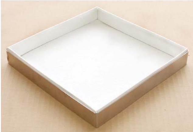
Square steel mold lined with ceramic fiber paper.
