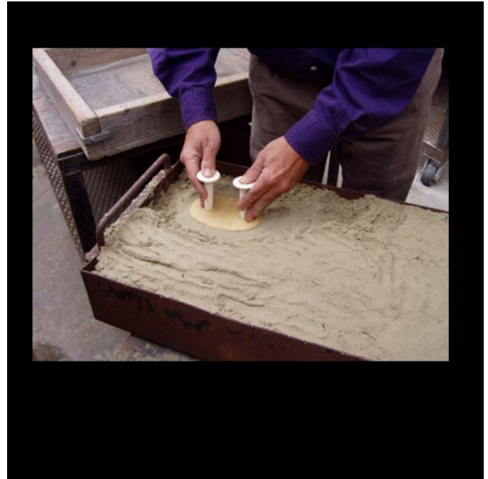
Pressing a casting shape into sand
