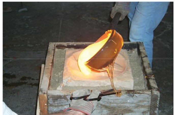
Pouring into a sand mold
