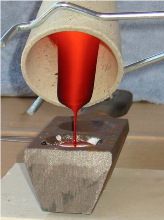
Pouring molten glass from a crucible into a mold
